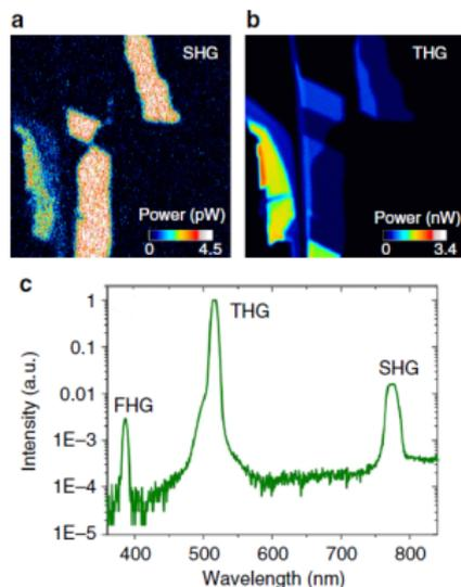
**Fig. 3** Multiphoton images of MoS<sub>2</sub> flakes. **a** SHG and **b** THG map of the flakes in Fig. 1a. **c** Optical spectrum of the nonlinear signal from 1L-MoS<sub>2</sub> with a peak irradiance  $\sim 30 \text{ GW cm}^{-2}$
