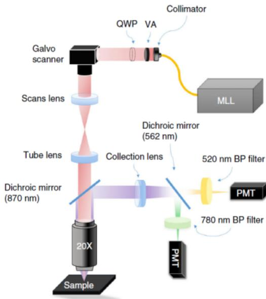
**Fig. 2** Schematic diagram of multiphoton microscope. MLL, linearly
