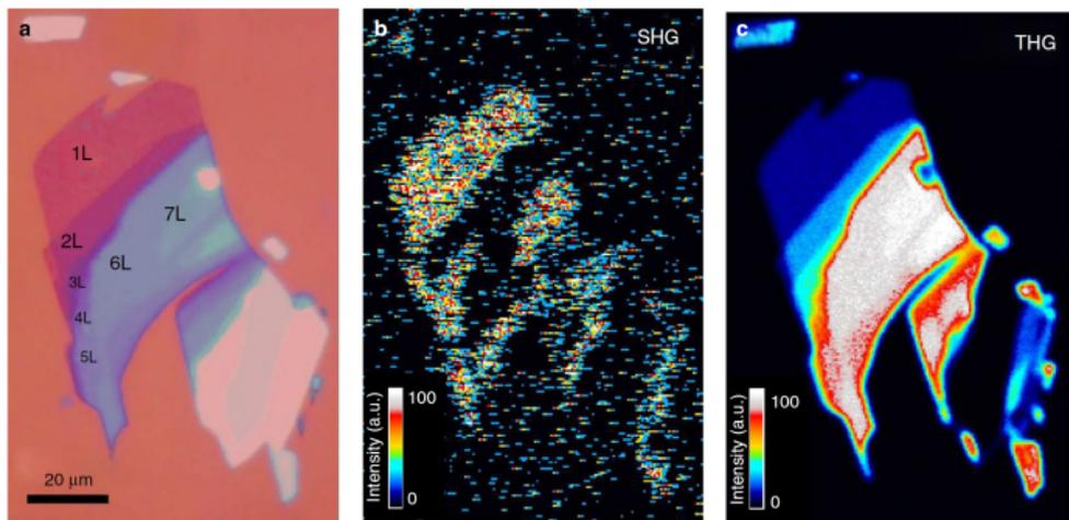
**Fig. 6** Optical and multiphoton images of few-layer MoS<sub>2</sub> flake. **a** Optical micrograph, **b** SHG, and **c** THG images of flake with few-layer areas under 1560 nm excitation
